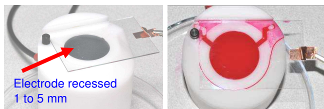
Figure 1. Standard cell with ITO-coated glass (left). Filled cell (right).
