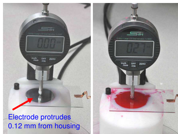
Figure 2. Special cell with ITO-coated glass in place (left). Cell with ink paste between electrodes (right).
