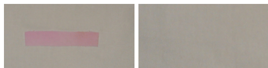
Figure 1: Cotton twill inkjet printed with Poly-R478 (left) before and (right) after washing.
