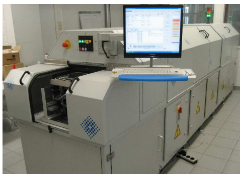
Fig. 5: Peptide printer for series production of peptide arrays. Designed and build in cooperation with KMS Automation GmbH.
