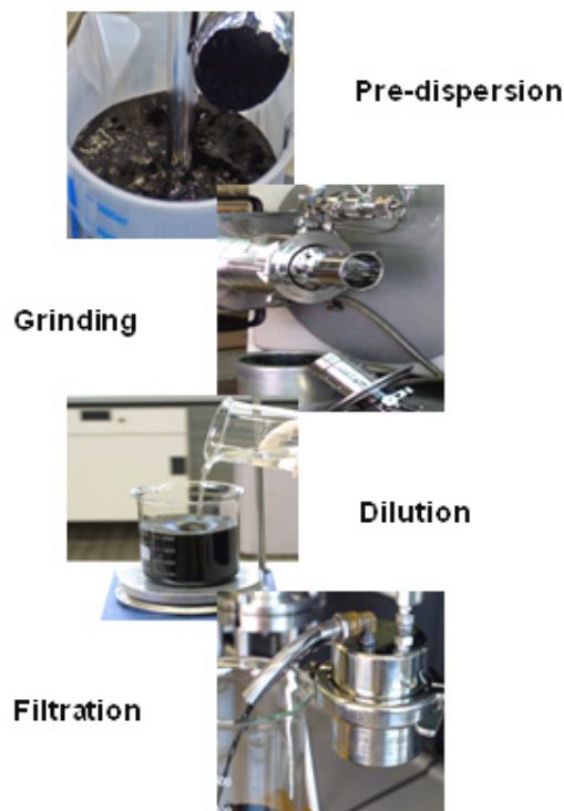
Figure 1: Process steps to prepare carbon black pigment dispersion for inkjet inks
