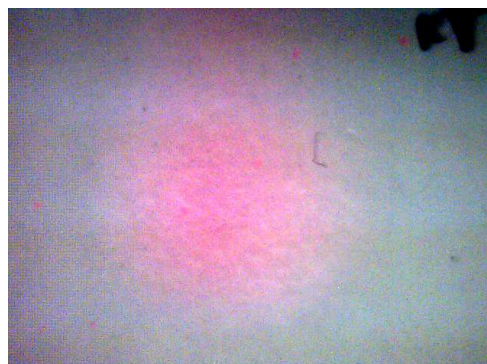
Figure 6: Picture of spray coated gelatin. (liquid level: 2.0 mm, applied voltage: 9.0 kV)
