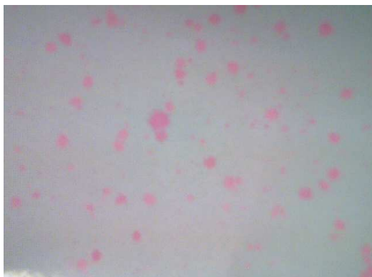
Figure 7: Picture of spray coated gelatin. (liquid level: 5.0 mm, applied voltage: 9.0 kV)
