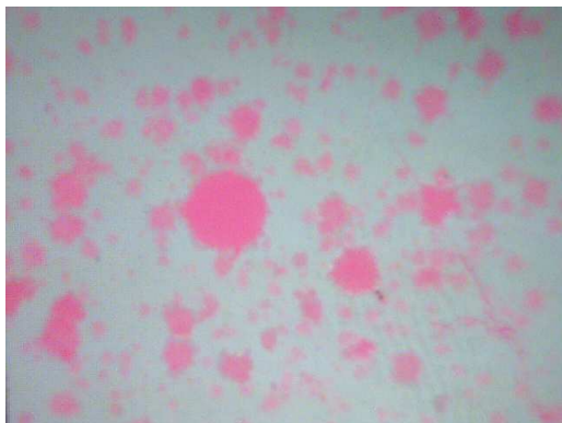
Figure 8: Picture of spray coated gelatin. (liquid level: 10.0 mm, applied voltage: 9.0 kV)
