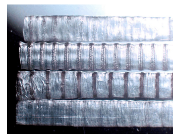
Figure 7 1mm diameter biosorbable conduits for peripheral nerve regeneration, fabricated using ink-jet printing methods. Nerve growth factor (NGF) is embedded in the conduit to stimulate direct growth.
