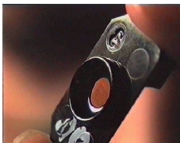
Figure 4 Disposable diagnostic test that contains up to 100 tests printed using ink-jet technology
