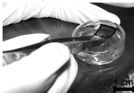
Figure 4. Fishing out a microsieve supported with a polymeric frame
