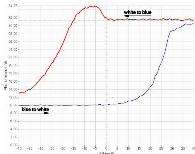
Figure 5. Electro-optical Curve for Blue / Reflective White EPD fluid (50 \mu m cell gap; CR = 3.2:1).
