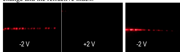
Figure 3. Photographs of the diffracted light image from the patterned ECD, showing reversible diffraction modulation at -2 V (colored) and +2V (bleached).
