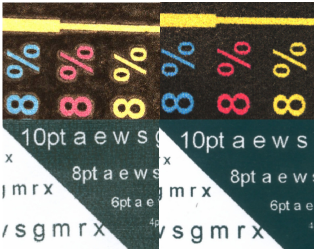
Figure 4. Inkjet printing results after surface sizing with cationic starch (left) and with AERODISP® WK7330 + cationic starch (2:1 with respect to solid, coating weight approx. 1 g/m 2 ).
