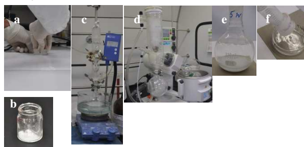
Figure 7. The steps using in preparing the sample. (a) the coating is scrapped off using a razor, (b) collected coating, (c) the sample is sequentially boiled, (d) the sample is concentrated, (e) concentrated sample and (f) the decanted liquid is filtered using a syringe filter.
