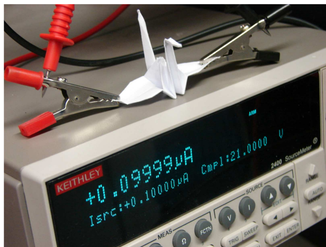
Figure 3. A sheet of paper with inkjet printed ionogel still demonstrates conductivity after being folded into an origami crane.
