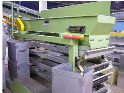
Figure 1. A typical vibration grading sifter. The grading sifter has four layers, in which the holes have different sizes. In precise, the higher the layer, the larger the holes. After vibrating a specific time, the tobacco leave are grouped into four classes, each of which has a specific range of sizes.
