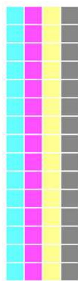
Figure 1. Test target for examining the uniformity of fading within test chambers.
