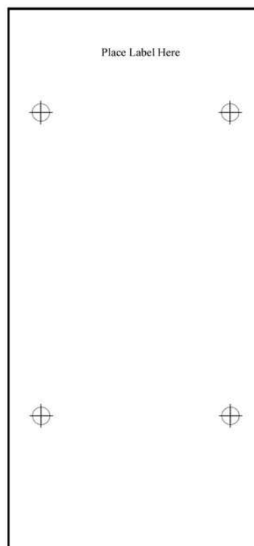
Figure 1. Example of unprinted test sample for evaluating media yellowing. Locating marks are outside the measurement area.
