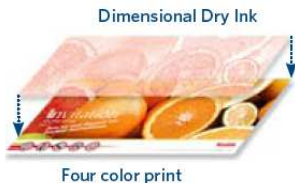
Figure 7: Dimensional Clear Dry Ink printed in the fifth station of a KODAK NEXPRESS SE-Class Digital Production Color Press creates a clear “raised” layer on top of a page element after fusing.
