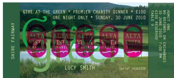
Figure 8: Red florescent security logo on a ticket digitally printed using Red Fluorescent Dry Ink in the fifth station of a KODAK NEXPRESS SE-Class Digital Production Color Press
