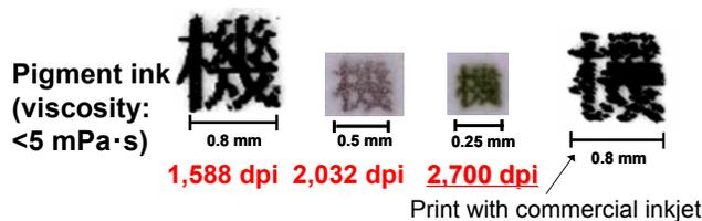
Figure 2: Print samples of Chinese character "mecha" by using the micro-drop injection and a commercial inkjet (liquid material: pigment ink)
