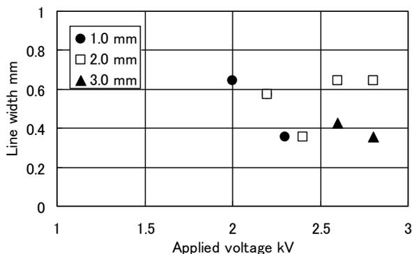
Fig. 12 Width of gelatin line when the applied voltage was changed. (density of gelatin: 1.0%)
