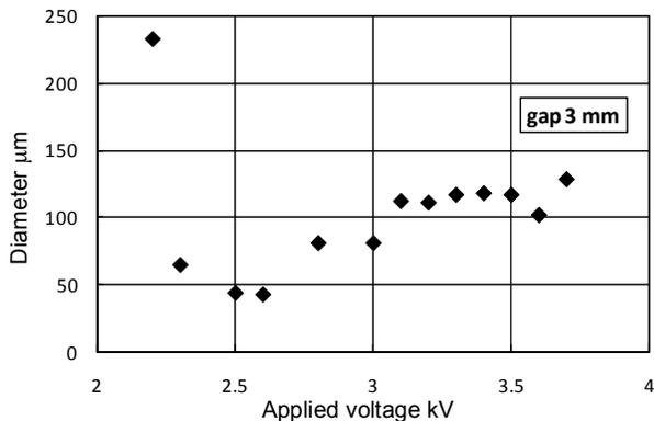
Fig. 11 Diameter of droplet of liquid with gelatin when the applied voltage was changed. (density of gelatin: 2.0%)
