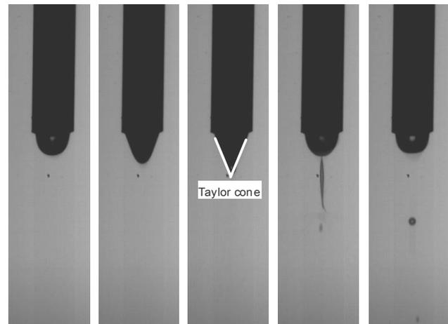
Fig. 9 Movie of droplet formation of liquid with gelatin. (density of gelatin: 1.0 %, applied voltage: 2.4 kV, air gap: 3.0 mm)
