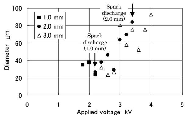
Fig. 10 Diameter of the ejected droplet when the applied voltage was changed. (density of gelatin: 1.0 %, parameter: air gap)
