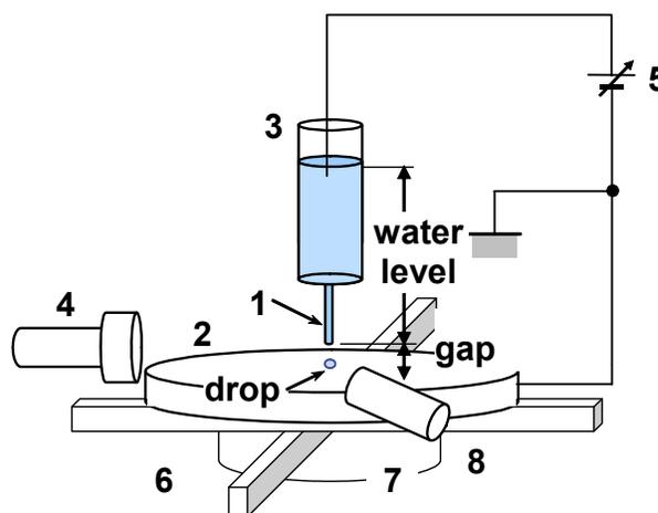
Figure 1: Experimental set-up of single nozzle inkjet system. (1: water pin electrode, insulative capillary tube filled with ink, 2: metal plate electrode, 3: ink tank, 4: high speed camera, 5: high voltage amplifier and function generator, 6: linear stages, x and y directions, 7: mechanical z-stage, 8: light)
