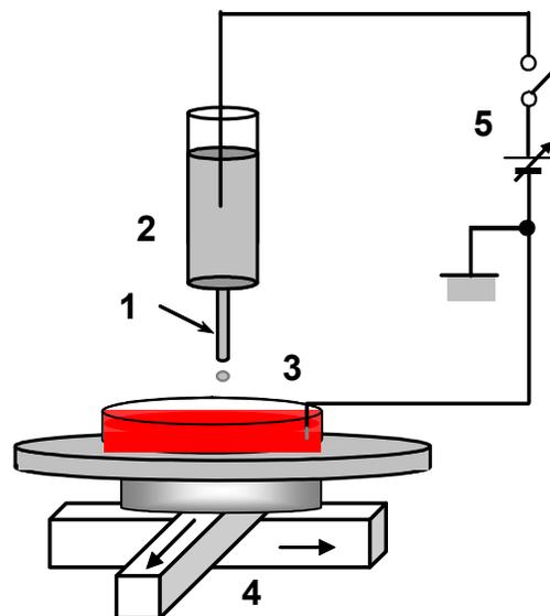
Figure 4: Experimental set-up of cell patterning utilizing electrostatic inkjet. (1: water pin electrode, insulative capillary tube was mounted at tip of syringe, 2: tank, filled with liquid of cells, 3: dish, filled with medium, 4: xyz linear stages, 5: DC high voltage power supply)
