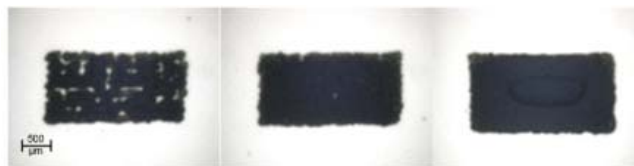
Figure 5. Influence of the drop spacing or resolution on structure appearance
