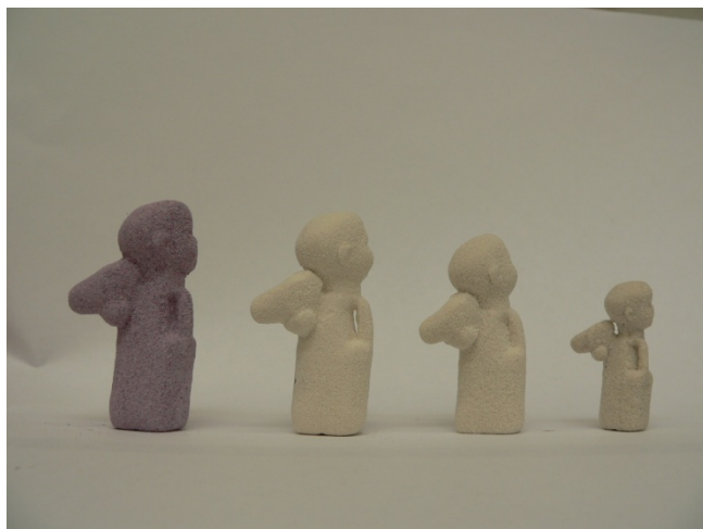
Figure 13. Ceramic 3D print size comparison unfired to 1250 deg C.
