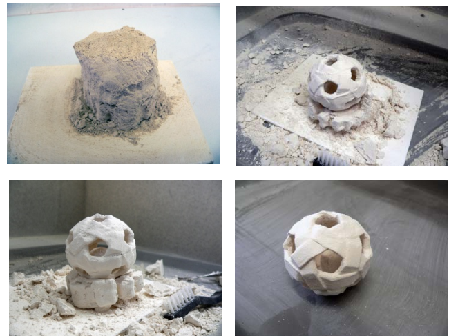
Figure 2. 3D ceramic printed from granulate
