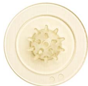
Figure 3. Anemone indicator in 3D printed photopolymer
