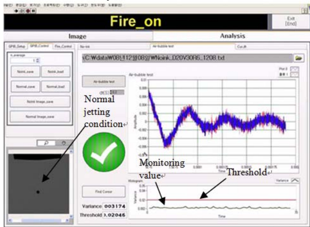
Figure 2. Software developed to monitor jetting status (normal condition) [8].
