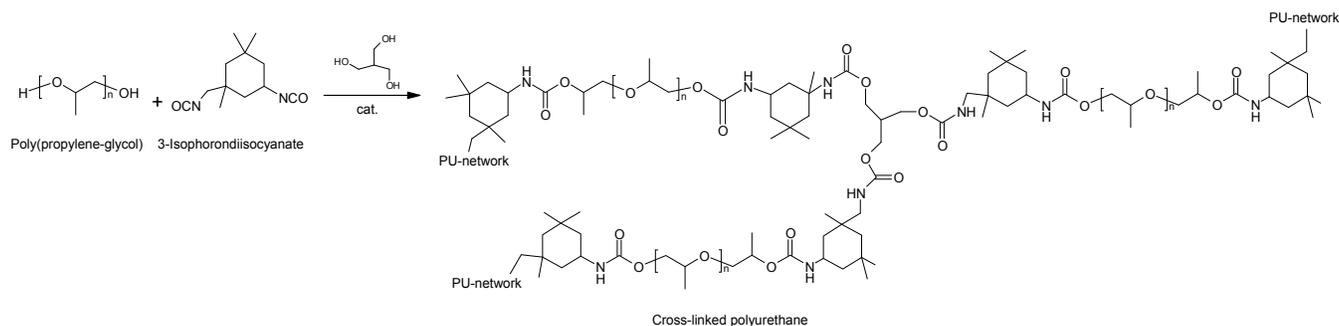
Figure 3. Schematic representation of the reaction scheme for the formation of polyurethanes from the reactants.
