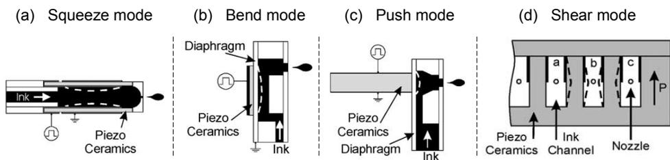
Figure 2. Different piezoelectric drop-on-demand technologies. Reprinted from ref. [13].
