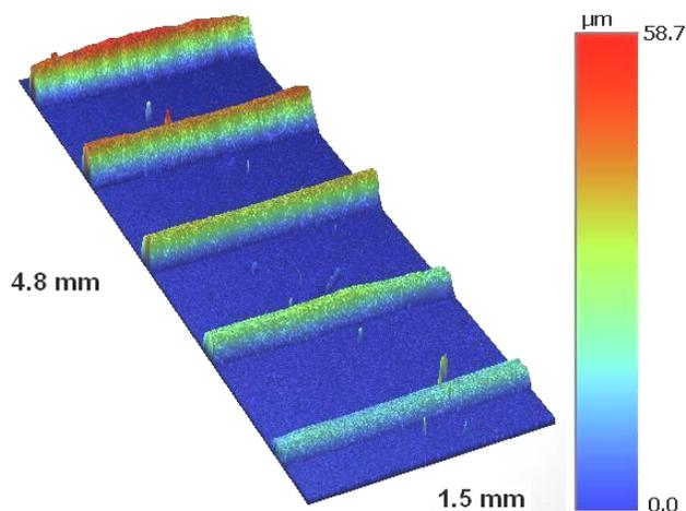
Figure 5. Five inkjet printed lines of *in-situ* formed polyurethane. From top to bottom, the parallel lines consist of an increased number of layers, where each layer consists of two print runs from both reactants. From top to bottom the number of layer decreases from 5 to 1, respectively.
