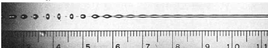
Figure 1. Break-up of a laminar flow-jet into a train of droplets, because of Rayleigh-Plateau instability. Reprinted from ref. [5].
