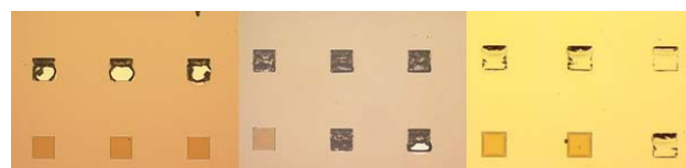
Figure 8 The transition from a cohesive to an adhesive failure mode with time in ink at T0, T1, and T16
