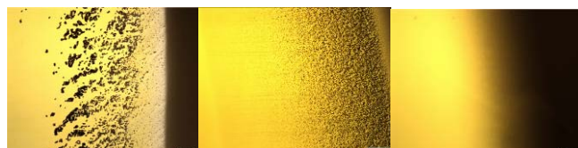
Figure 4: Light microscopic images (200x) of the transition from a black to a yellow ink drop. The flocculation tendency (from left: strong: GB-B, moderate: GB-A, no: GB-C) correlates with inter-color bleeding properties after printing.
