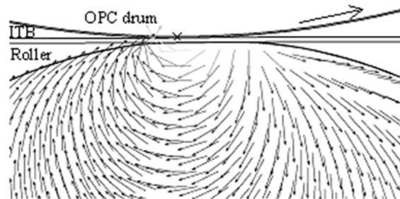
Figure 8. Calculation result of electric field in transfer roller when offset is 0.5mm
