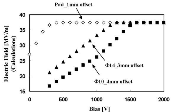
Figure 12. Relationship between bias and maximum transfer electric field
