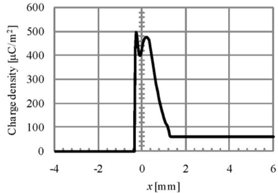
Figure 7. Calculation result of charge density in ITB when offset is 0.5mm
