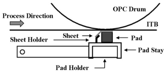
Figure 2. Cross-section of pad transfer unit
