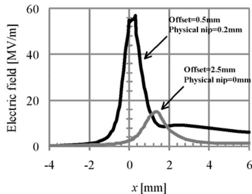
Figure 6. Electric field between OPC drum and ITB
