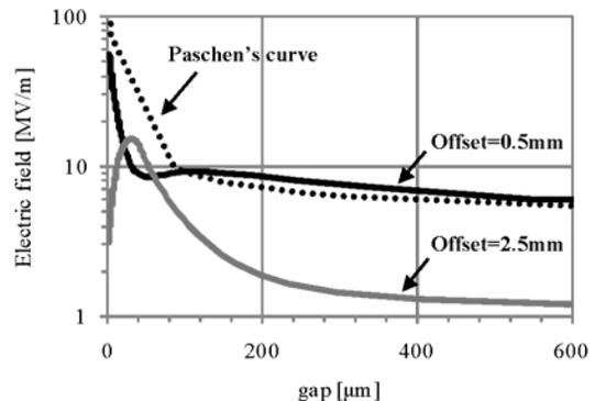
Figure 9. Electric field between OPC drum and ITB in downstream nip region
