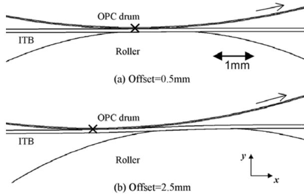
Figure 4. Calculation results of nip shape
