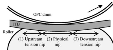
Figure 5. Schematic illustration of nip region
