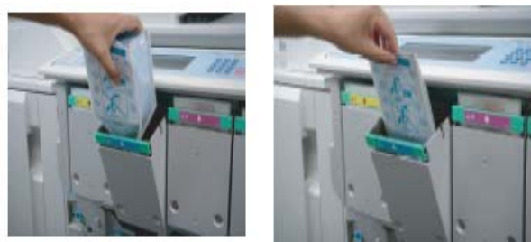
Figure 7. Auto volume reduction cartridge in Multifunction color copier
