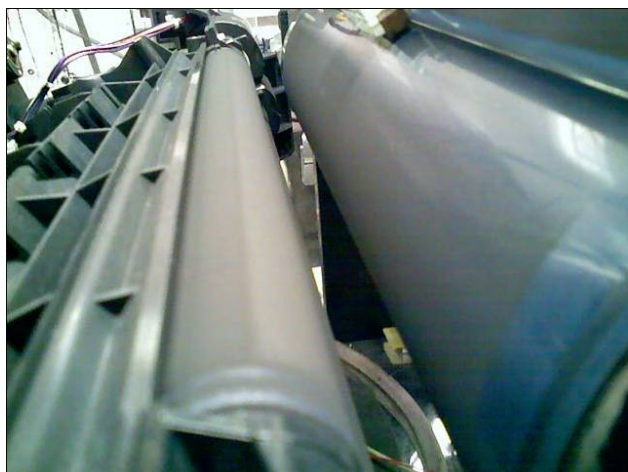
Figure 5: Experimental apparatus to verify the effectiveness of MC-SJD. The donor roll is to the left, and the aluminum receiver roll is to the right. An AC field, as either a simple jumping waveform or the move complex MC waveform, is applied between the two rolls. If the donor has a negative DC bias, negative toner tends to develop on the receiver. If the donor is positively biased, toner tends to return to it.
