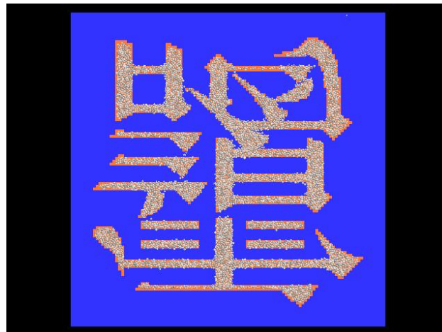
Figure 4: Simulated development of a 4-point Kanji character using 4 \mu m toner. The simulation was terminated after approximately 2 ms of run time. As this is considerably less than a typical nip's transit time, the image has not yet fully developed.
