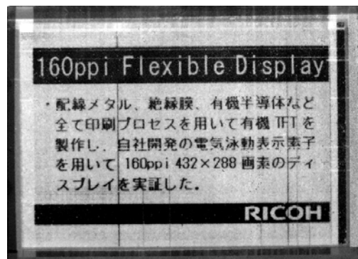
Figure 7. A 160 ppi EPD driven by all-printed OTFT backplane on flexible substrates
