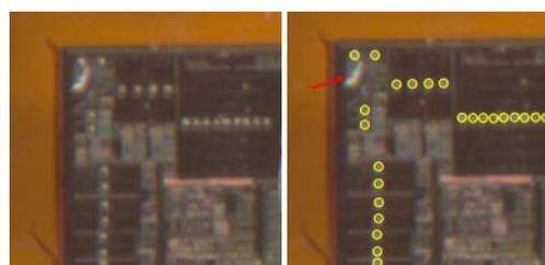
Figure 2. Closer look at the module. The wiring targets are the golden pads near the edges of the IC. They are detected automatically by the front end, as seen on the right. Note, that the pad pointed by the red arrow is covered by dust, and can not be found by the front end.
