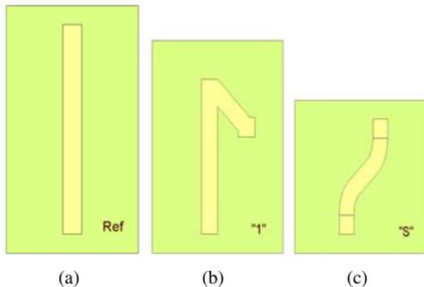
**Figure 8.** Line geometries used in the electrical performance simulations. Original line with no component displacement (a), misalignment corrected using erase-and-redraw algorithm (b), and misalignment corrected using smooth correction algorithm (c).
