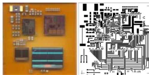
Figure 1. A sample multi-IC module (left) ready for printing the connections (right).
