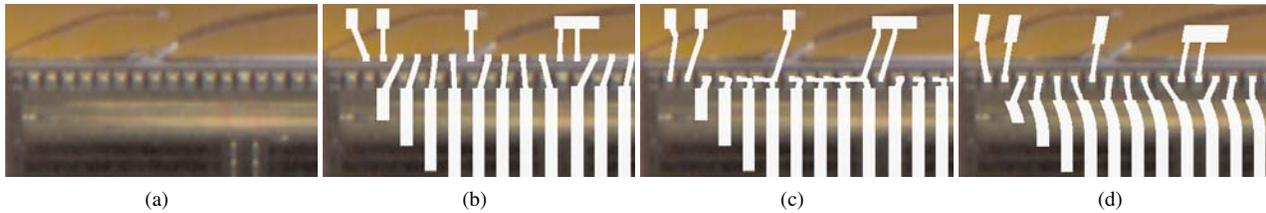
**Figure 7.** Original module ready for printing (a), and the simulated printing result without correction (b). The simulated result with erase-and-redraw correction (c) and the result with the smooth correction (d).
