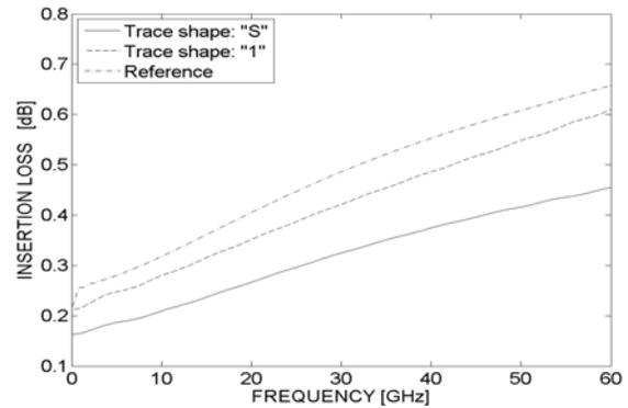
**Figure 9.** Simulated insertion loss for the three different line geometries considered.
