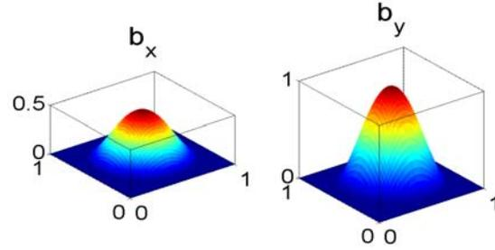
**Figure 4.** An example of smooth bump created with piecewise biquadratic polynomial with  $(x, y) = (0.5, 0.5)$ ,  $\boldsymbol{\delta} = [0.5 \ 1]^T$  and  $s = 0.4$  (and  $R = 0.45$ ).
