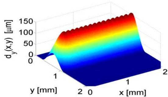
**Figure 6.** A part of the displacement map used in Figure 7 (only vertical displacement shown; the horizontal direction map is similar but with negative peaks as the displacement is directed from right to left).
