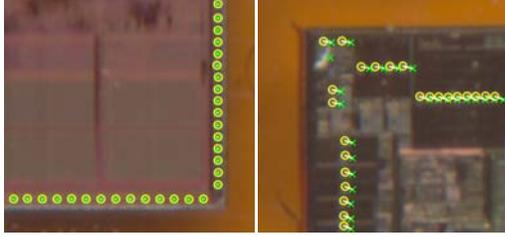
**Figure 3.** Pairing the design data with the detection result. The figures show the match with the true locations of the pads. The figure on the left shows a part of the calibration IC, and the one on the right is a part of another IC.
