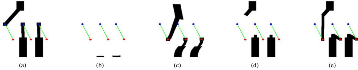
**Figure 5.** Illustration of the correction process. The figure (a) shows the connection points and connectors before correction. In (b), the wire ends have been erased and in (c) redrawn using the proposed method. For comparison, Figures (d) and (e) show the erasing and redrawing phases using the old method.
