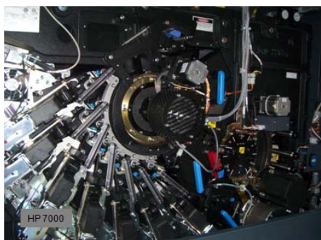
Figure 6. HP Indigo Series III marking engine.
