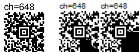
Fig. 1. Example of original and damaged Aztec Code 2D barcodes (ch=648 indicates maximum bits to use for encoding characters). Original size was 20 x 20 mils per module. Payload is 456 out of 648 payload bits (30% ECPSA). Images show no damage (left), 12.5% damage (center) and 25% damage (right).
