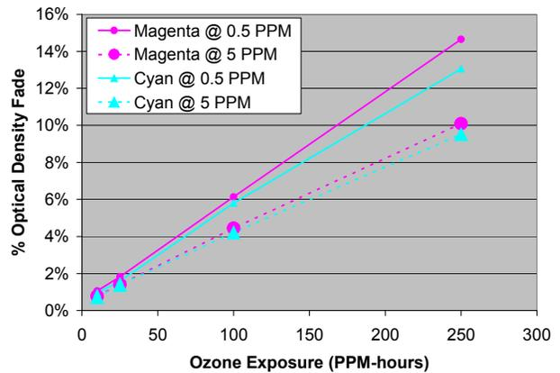
**Figure 2. System G6 Cyan and Magenta Patch Fade For 0.5 PPM and 5 PPM Ozone Test Concentrations.**
