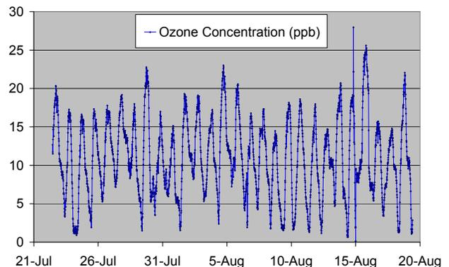
Figure 1. Ozone Measurements Collected During Ambient Ozone Test (in ppb). Four Week Window Shown is Representative of Entire Three Month Test.
