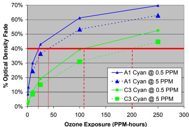
Figure 3. Systems A1 and C3 Cyan Patch Fade For 0.5 PPM and 5 PPM Ozone Test Concentrations.
