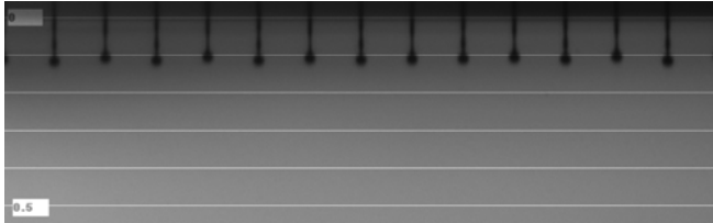
Figure 5. Single cycle, 2-phase operation of 42 pl drops (7 drops each at 6pl) emerging from a 180 dpi nozzle and shared wall array.
