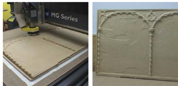
Figure 6. Milling process and table sample
