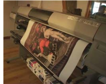
Figure 8. Papelgel material being printed in a HP Designjet 5500 as any other conventional photo media
