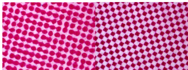
Figure 10: 50% magenta dots comparison. Left one was printed by the Indigo press. Right one was printed by the Speedmaster press.
