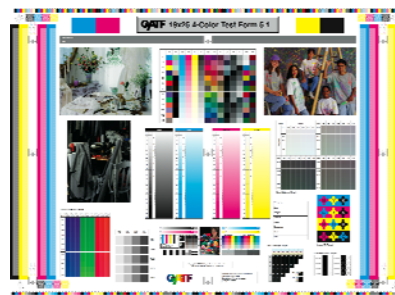
Figure 1: GATF 19 by 25 inches test form for the Heidelberg Speedmaster CD74 press.
