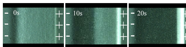
Figure 5. Electrophoresis of Negative Charged Particle Moving to Positive Electrode (left is negative electrode)
