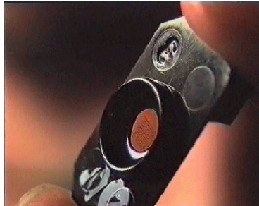
Figure 3 Disposable diagnostic test that contains up to 100 tests printed using ink-jet technology
