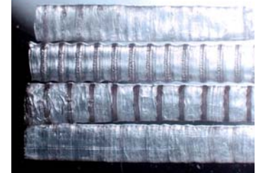
Figure 7 1mm diameter biosorbable conduits for peripheral nerve regeneration, fabricated using ink-jet printing methods. Nerve growth factor (NGF) is embedded in the conduit to stimulate direct growth.
