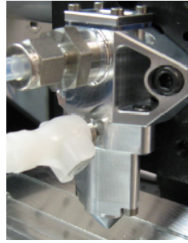
Figure 7: Prototype Bus Bar Printing Head – three bus bars are printed simultaneously.
