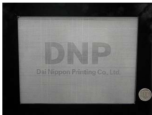
Figure 6. A QR-LPD driven with printed AMOTFT array consist of 80 dpi, 640x480 pixels (10inch VGA).
