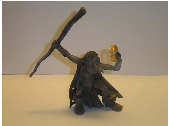
Figure 2: A fairy made in PA12-material by the SMS-process.
