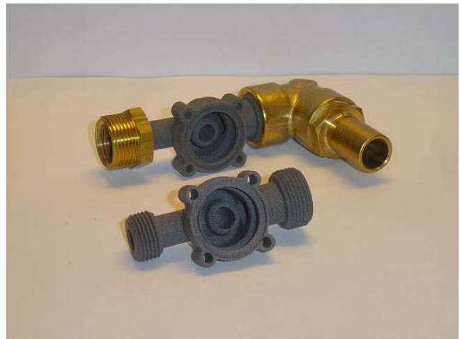
Figure 3: Two pump-houses made of PA12-material by the SMS-process. One of them shows the fit of the SMS-part to the two threaded metal tubings.
