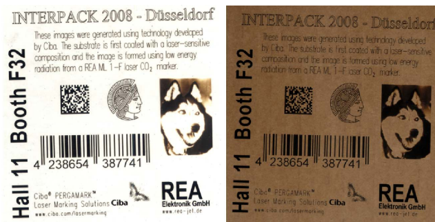
Figure 2. Images produced at low laser power on paperboard substrates demonstrate high resolution, high contrast codes which can be achieved on packaging treated with laser active inks or coatings.
