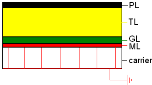
Figure 2. Schematic cross section of the OPC. PL represents a protective layer of about 0.2 \mu\text{m} , TL the transport layer of about 10 \mu\text{m} , GL the generation layer of about 0.5 \mu\text{m} and ML the metal layer of about 0.1 \mu\text{m} . The ML is grounded via perforations in the polyester carrier belt.
