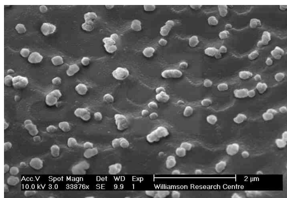
Figure 3: Cryo-ESEM image Anthraquinone Magenta H.110 300 and dye-copolymer (MMA/EHMA/MAA = 47.5/35/17.5) nanoparticles at 1:3 w/w ratio.
