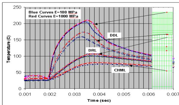
**Figure 7.** Effects of Young's Modulus of CHML on thermal history of the thermal dye donor and thermal dye receiver.
