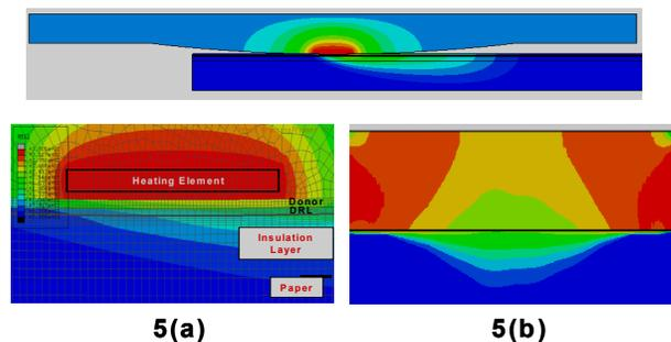
Figure 5(a). Temperature distribution in the thermal media and areas close to the heating element. Figure 5(b). Dye distribution in the thermal media.
