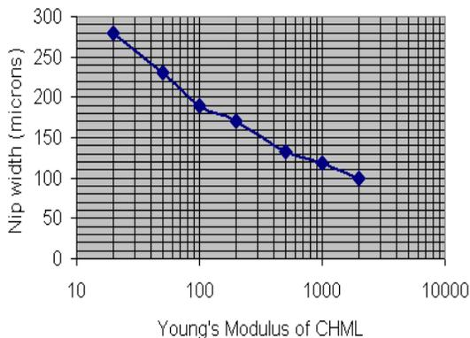
**Figure 6.** Nip width vs. Young's Modulus of CHML (simulated at ambient temperature).
