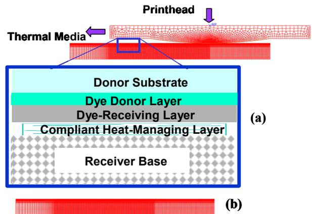
Figure 4. Typical finite element mesh for (a) coupled thermal-structural nip analysis and (b) coupled thermal-dye diffusion analysis.
