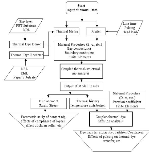
Figure 2. Flow chart of the coupled thermal-mechanical-dye diffusion analysis.
