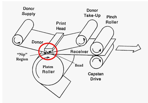
Figure 1. A typical thermal printing scheme.
