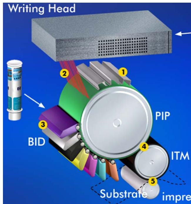
Figure 1. HP Indigo digital press – printing engine schematic
