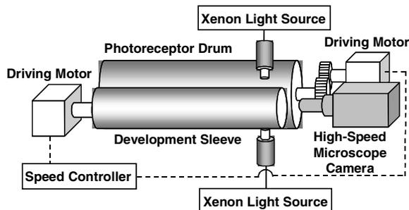
**Figure 2.** Experimental setup to observe the dynamic behavior of carrier and toner particles in the development area with the high-speed microscope camera.
