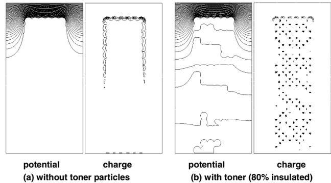
**Figure 9.** Distributions of steady-state potential and charge density in conductive carrier chain with and without insulative toner particles.
