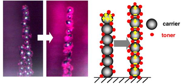
**Figure 7.** Photograph of chains to which the toner particles adhered and conceptual drawing of charge distributions in the chains that contain rare and sufficient number of toner particles.
