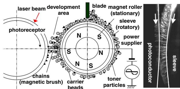
Figure 1. Schematic drawing of two-component magnetic brush development system in electrophotography (left) and photograph of magnetic brush in the development area (right).
