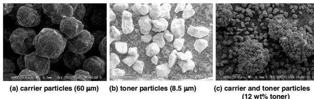
**Figure 3.** SEM photographs of carrier particles, toner particles, and mixture of both particles.
