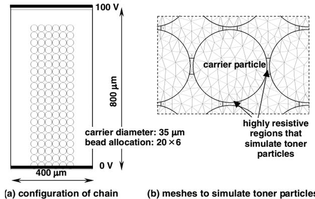
**Figure 8.** Calculation conditions: configuration and dimensions of the calculation domain and meshes to simulate the presence of toner particles.
