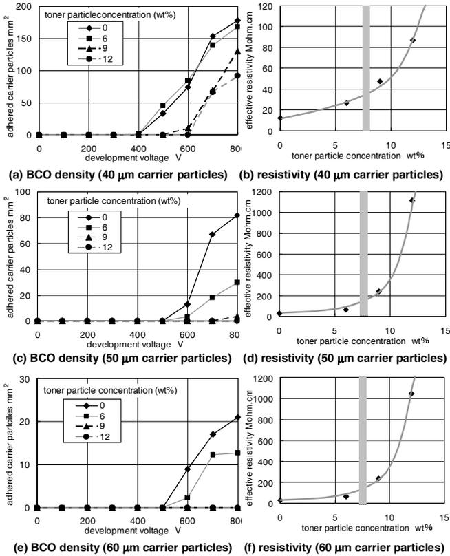
**Figure 6.** Number density of adhered carrier particles on the photoreceptor drum (left) and the effective resistivity of a mixture of both carrier and toner particles (right). Confirm that the maximums of the ordinates in (c) and (e) are 50% and 15% of that of (a), respectively.
