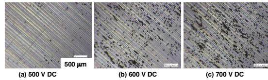
**Figure 5.** Examples of photographs of the drum surface taken after the development process (diameter of carrier particles: 40  $\mu\text{m}$ , toner particle concentration: 6 wt%).
