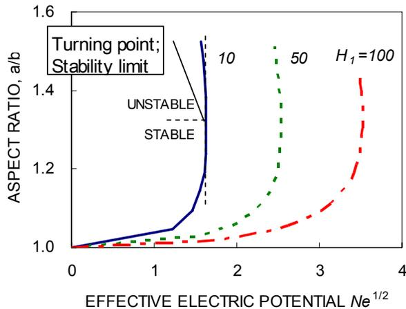
Fig. 4 The effect of a distance  $H_1$  from the bottom plate on the aspect ratio.  $G = 0$ ,  $H_2 = 100$ ,  $L = 100$ ,  $D = 0$ .
