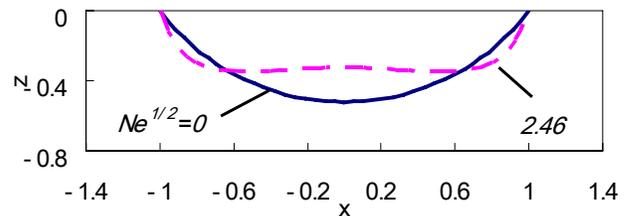
Fig. 7 Evolution of drop shapes with effective potential when  $G = 0$ ,  $H_1 = 10$ ,  $H_2 = 100$ ,  $L = 100$ ,  $D = -0.7$ .
