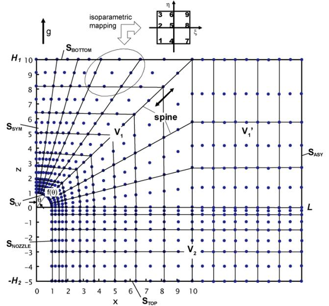
Fig. 3 An example of physical domain of calculation divided into finite elements. The figure above shows isoparametric mapping from/to physical domain to/from calculation domain.
