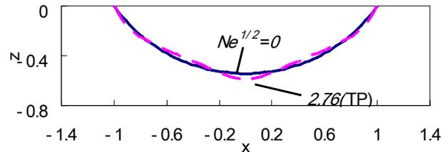
Fig. 6 Evolution of drop shapes with effective potential when  $G = 0$ ,  $H_1 = 10$ ,  $H_2 = 100$ ,  $L = 100$ ,  $D = -0.65$ .
