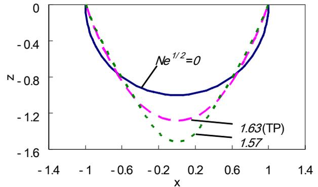
Fig. 5 Evolution of drop shapes with effective potential when  $G = 0$ ,  $H_1 = 10$ ,  $H_2 = 100$ ,  $L = 100$ ,  $D = 0$ .
