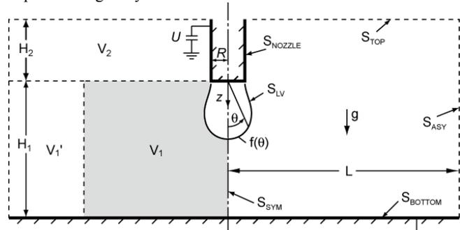
Fig. 1 Axisymmetric drop hanging from a nozzle in the presence of an electric field
