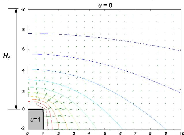
Fig. 8 Electrostatic field surrounding a nozzle when  $G = 0$ ,  $H_1 = 10$ ,  $H_2 = 100$ ,  $L = 100$ ,  $D = -0.7$ ,  $Ne^{1/2} = 2.46$ . \* Limited area is shown.
