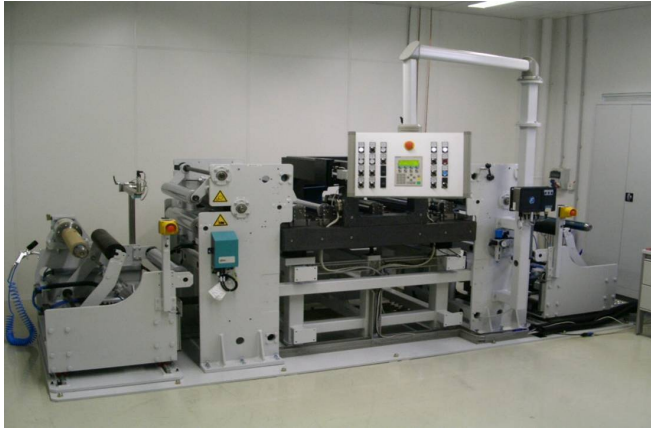
Figure 9. Roll-to-roll standard laser machining tool for flexible substrates
