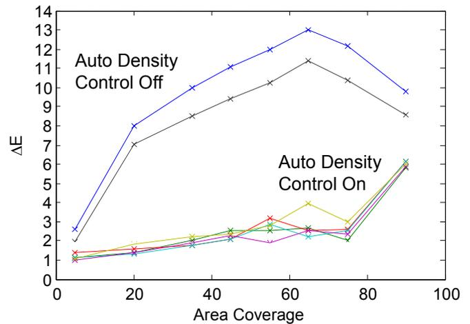
Figure 8 – Maintenance of uniformity over long runs.
