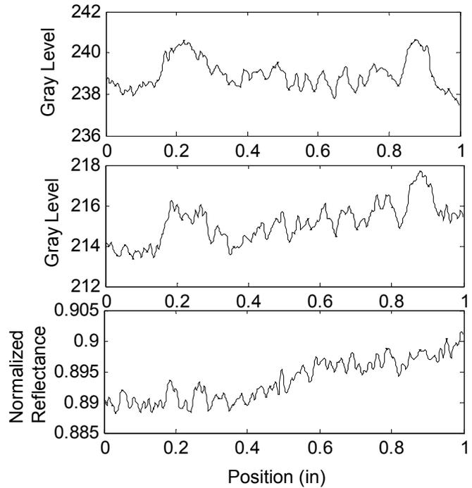
Figure 4 – Section of patch profiles: Top – Bare photoreceptor calibrate profile, Middle – 12.5% area coverage halftone calibrated profile, Bottom – 12.5% area coverage halftone normalized profile.
