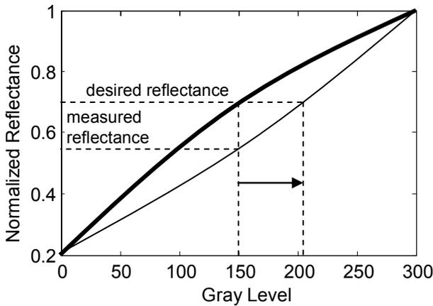
Figure 6 – Schematic illustration of streak compensation.
