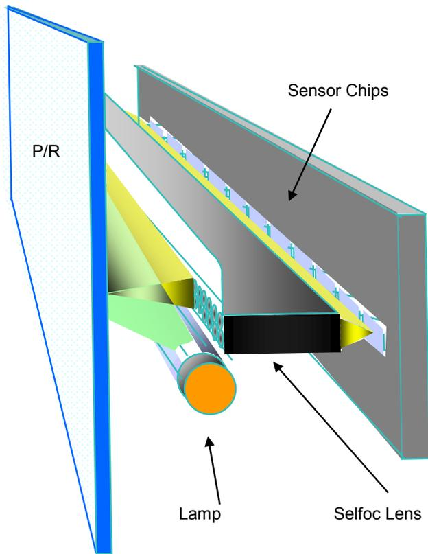
Figure 2 – Inline full width array imager
