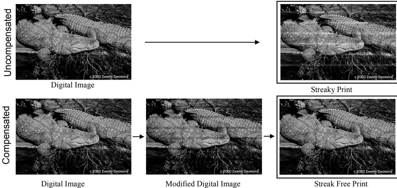
Figure 1 – Top: illustration of perfect digital image resulting in streaky print. Bottom: Illustration of modification of original digital image to produce streak free prints. Auto Density Control determines the correction automatically without making prints.
