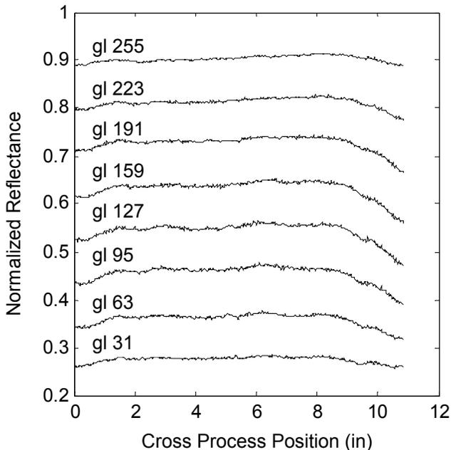
Figure 5 – Normalized uniformity profiles at different gray levels.
