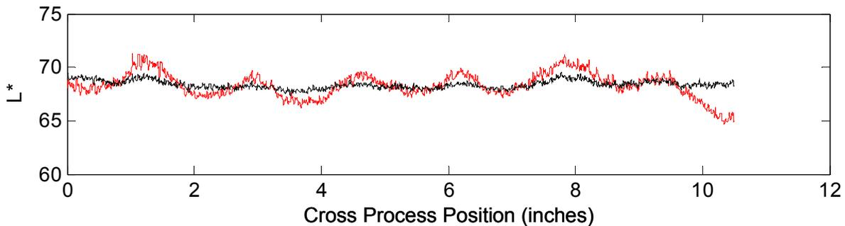
Figure 7 – Experimental demonstration of the elimination of streaks by the application of auto density control.
