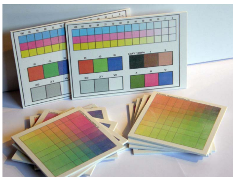
Figure2. 3D prints used for measurements, non-infiltrated sample presented
